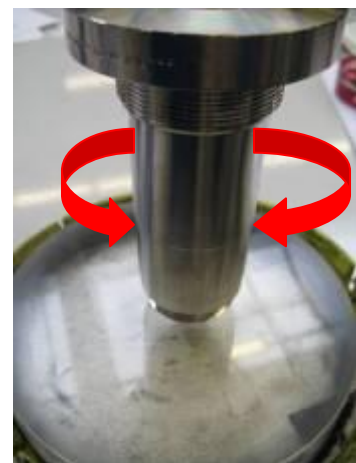
Fig. 5 Re-lapping the nozzle and the disc
