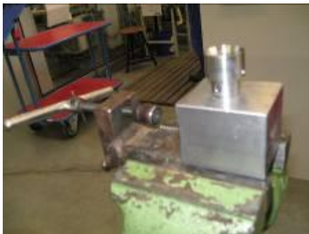
Fig. 3 Assembly apparatus for O-ring discs
