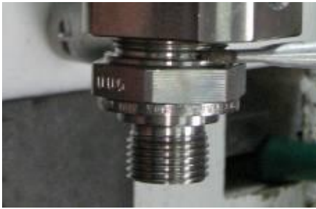
Fig. 4 Assembly of the inflow device
