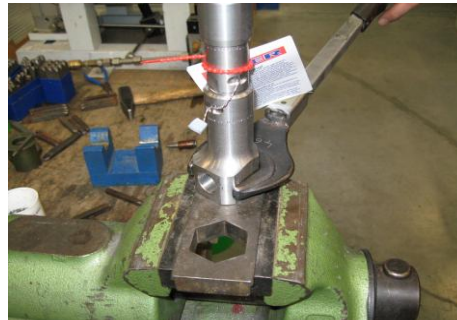
Fig. 5 Assembly of the outflow device with a fixed torque specification
