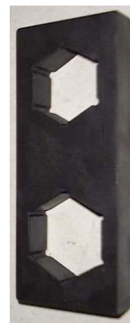
Illustration 1: Assembly aid for hexagonal inflow devices
