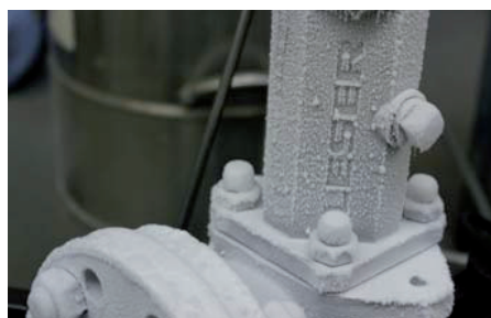
Fig 1: Test setup for cryogenic tests on spring loaded safety valves.
