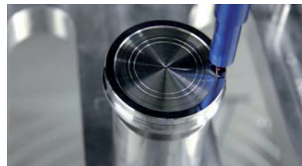
Fig 2: With LESER Nanotightness Technology, a new manufacturing concept, the tightness requirements of API 527 for gases are exceeded by 50 percent.
