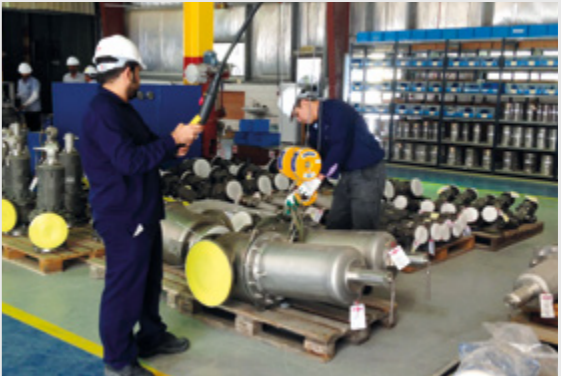
Binzagr assembly for LESER Safety Valves in Saudi Arabia
