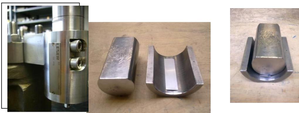
The nameplate has to be placed with its inscription upside down in longitudinal direction in the punching tool (cavity). The required form is achieved by 2-3 times manually hammering onto the plunger.
