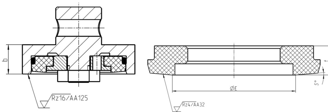
**Figure 4. Sealing plate disc**
