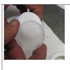
Place the glas sealing plate on the bellows with the rough side showing to the bellows. Screw on the lifting aid by hand until stop so that the sealing plate is clamped.
