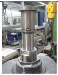
Shift the snap ring loosely onto the spindle. Place the spindle cap on top of the spindle and lock it with the pin. Position the snap ring in the groove of the spindle cap to lock the pin.
