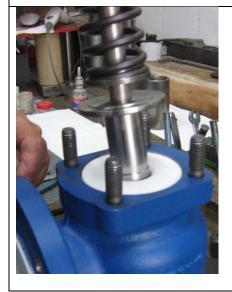
Fit the preassembled spindle-/spring-components carefully into the bellows within the body.
