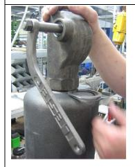
Lubricate and apply lifting device and gaskets. Hereby, place the lever in a position that the lifting fork is pushed away from the spindle cap (see photo).
