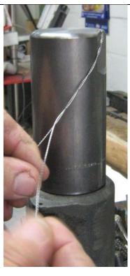
Link the sealing hole of the cap / lifting-device to the sealing hole of the bonnet, hereby twirl the wires clockwise and close to each other.
