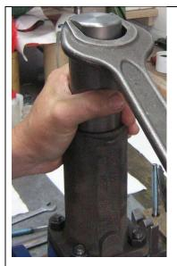
Place the H2-cap onto the Bonnet and tighten it with a wrench.
