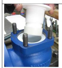
Turn the body again (inlet side showing downwards and fix the body to the table (e.g. on the test bench).
