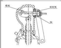
Adjust the excentric hole of the adapter so that the top of the spindle cap is in line with the top of the lift indicator (see figure).
