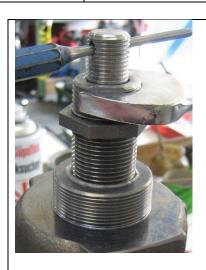
Secure the spindle against rotation with a drift pin.
