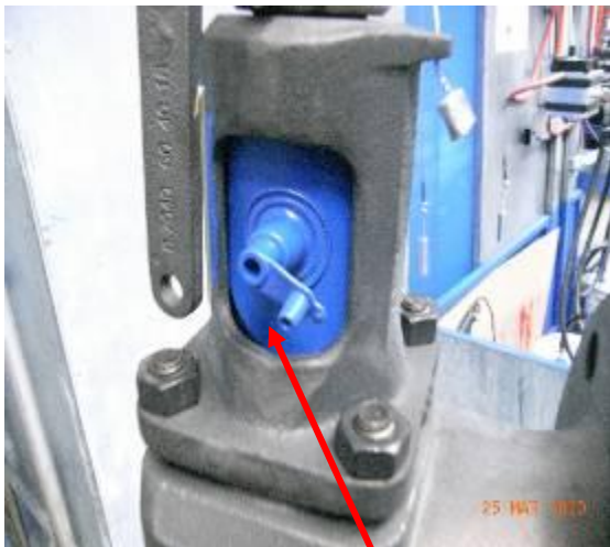
Figure 6-1: Protective cap for open bonnet
