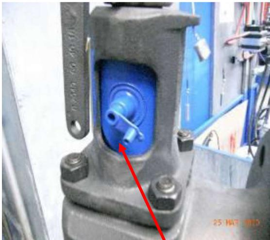
Figure 6-1: Protective cap for open bonnet
