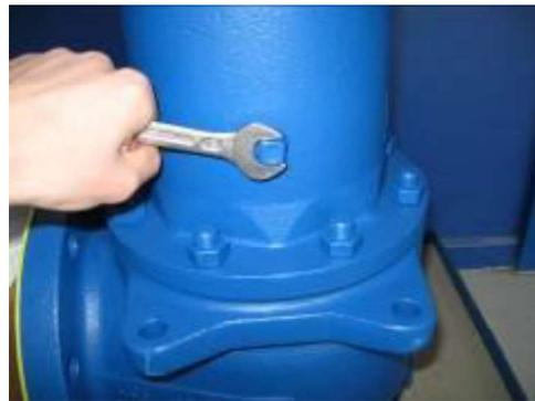
Fig. 2 Sealing the drain hole
