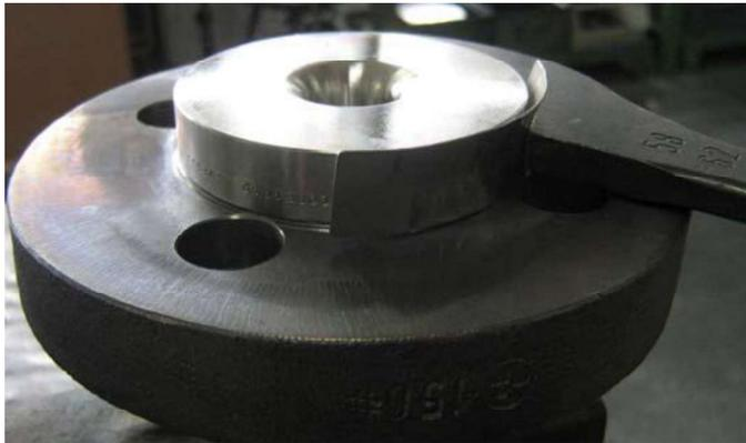
Fig. 3 Installing the nozzle
