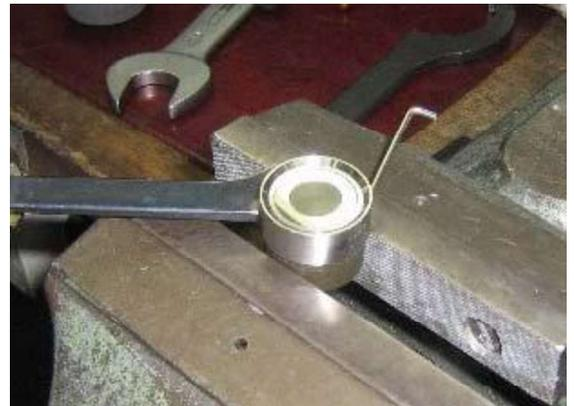
Fig. 4 Installing the snap ring
