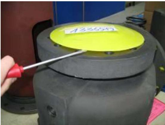
Fig. 3 Lifting the protective cap
