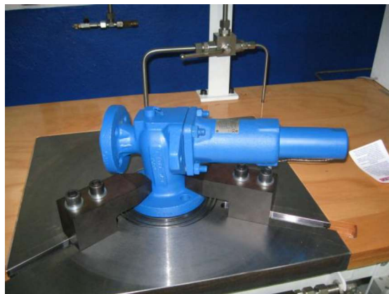
Fig.: 21: Clamping on the valve
