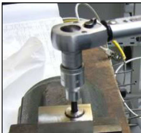
Figure 7: Allen key with torque wrench
