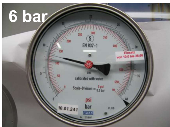
Fig. 22: Test pressure 6 bar
