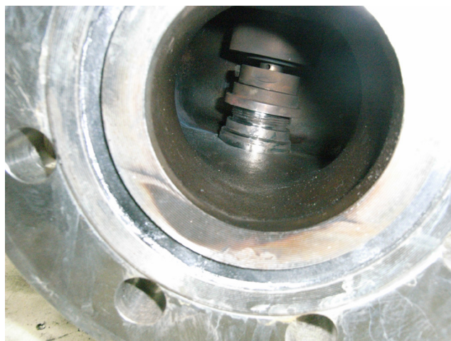
Figure 3. Inner body of LESER safety valve after two years of usage – no signs of crystallisation or corrosion.
