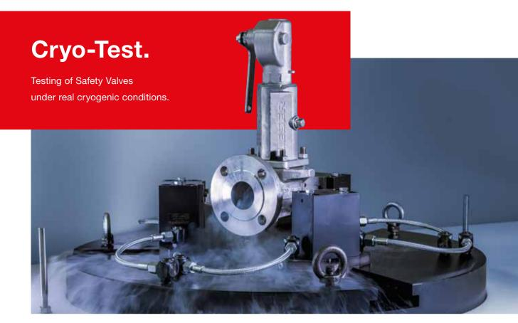
Challenging conditions are expected in LNG liquefaction and regasification plants: Low temperatures down to -164 °C / -263 °F and high pressures up to 155 bar/ 2248 psi. It is important for plant operators to know that their safety valves are tight and will work reliably, even under these extreme operating conditions.
